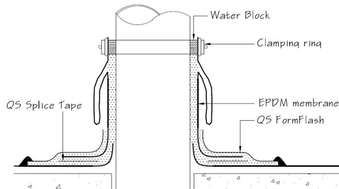
Figure 8. Schematic diagram of the "safety pleat" on the biogas collection wells
