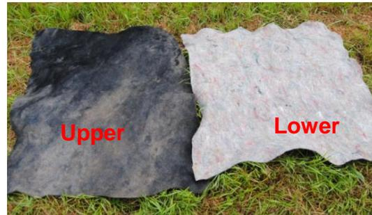
Figure 12. EPDM geomembrane and color difference between the upper and lower geotextile
