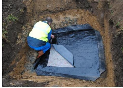
Figure 11. Taking samples of the EPDM geomembrane
