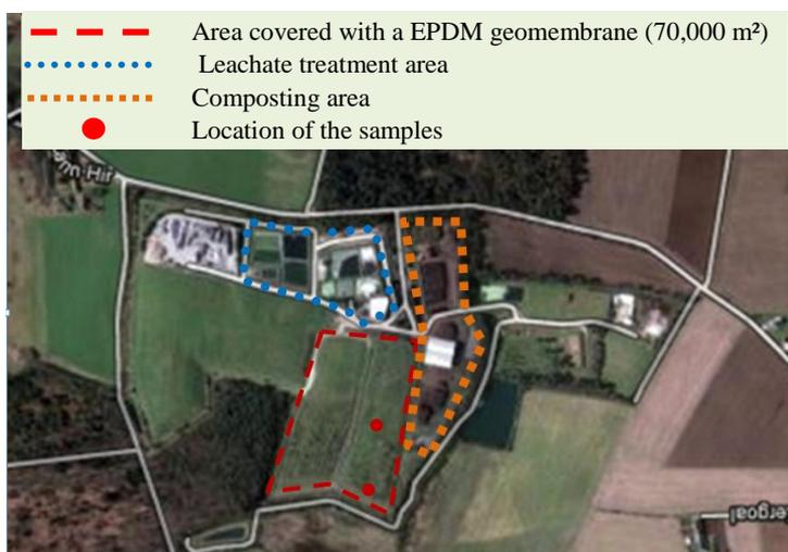
Figure 1. Aerial view of the Lann Hir landfill during covering work
