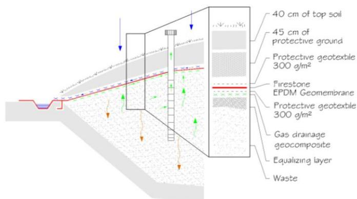
Figure 3. Schematic diagram of the Lann Hir landfill cover
