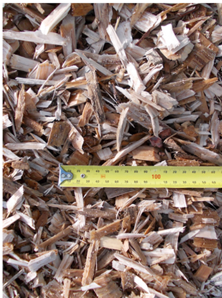
Fig. 2. Untreated woodchips ( Pinus radiata ) used as source of electron donor in the Tatuani bioreactor. Scale in the tape measure in mm.
