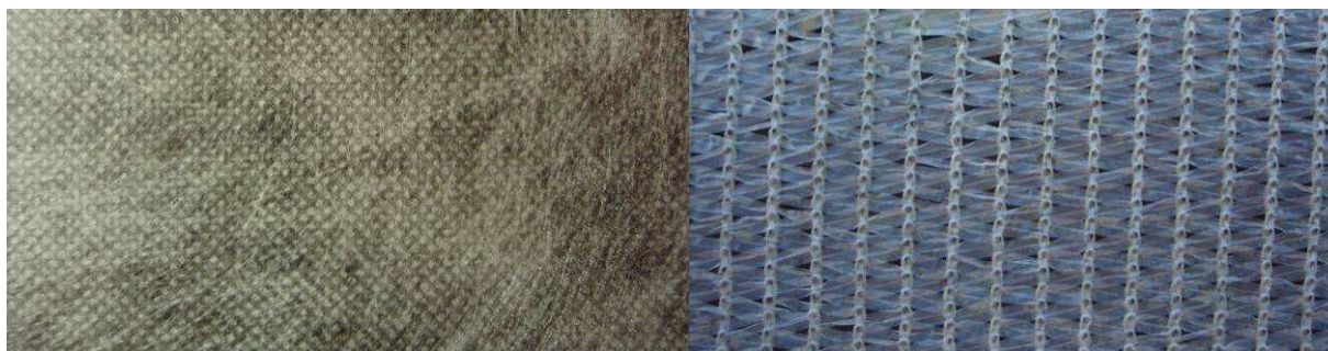
Figure 1. Spun-bonded frost cloth (left) and Mikroclima™ knitted frost cloth (right).
