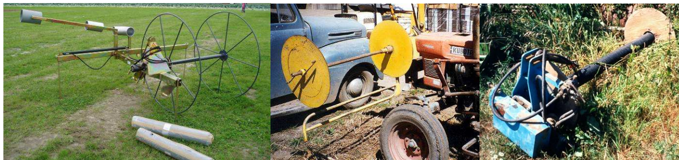
Figure 8. Three examples of floating crop cover handling systems all using removable bobbins.
