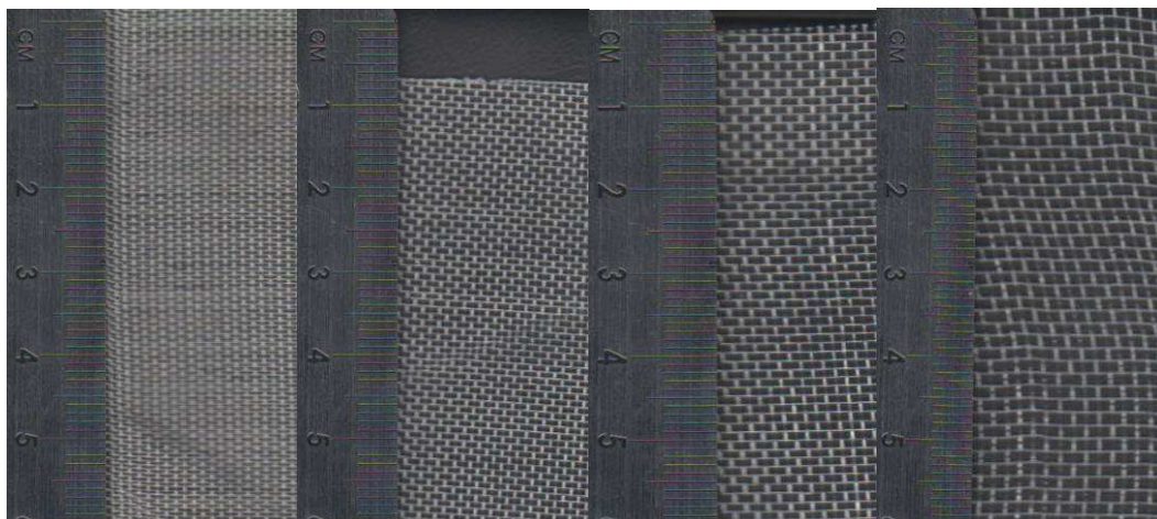
Figure 2. From left to right, four grades of mesh crop covers, 0.3 mm (thrips), 0.6 mm (aphids), 0.8 mm (flea beetle), and 1.3 mm (root fly) hole sizes.
