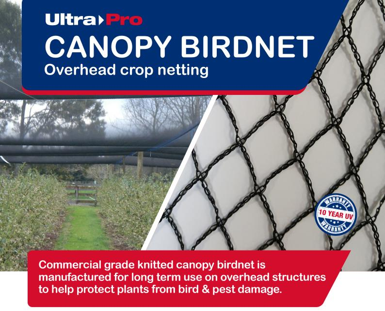
Canopy birdnet has a 16mm mesh size and is designed to be fixed to overhead cables for covering large areas of crops where bird & pest protection is required. Canopy birdnet will also give some protection from wind. Use cosio CFlex shackles, or cable clip lock to attach birdnet to wire or cables. When cutting birdnet to length allow an extra 25-30% this will ensure the birdnet is the correct length when fixed at the stated width.
