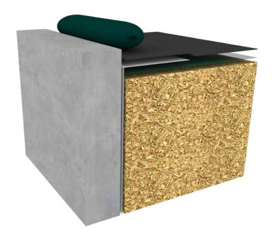
Lateral detail of a silage heap
